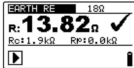
Figure 5.40: Example of earth resistance measurement result
